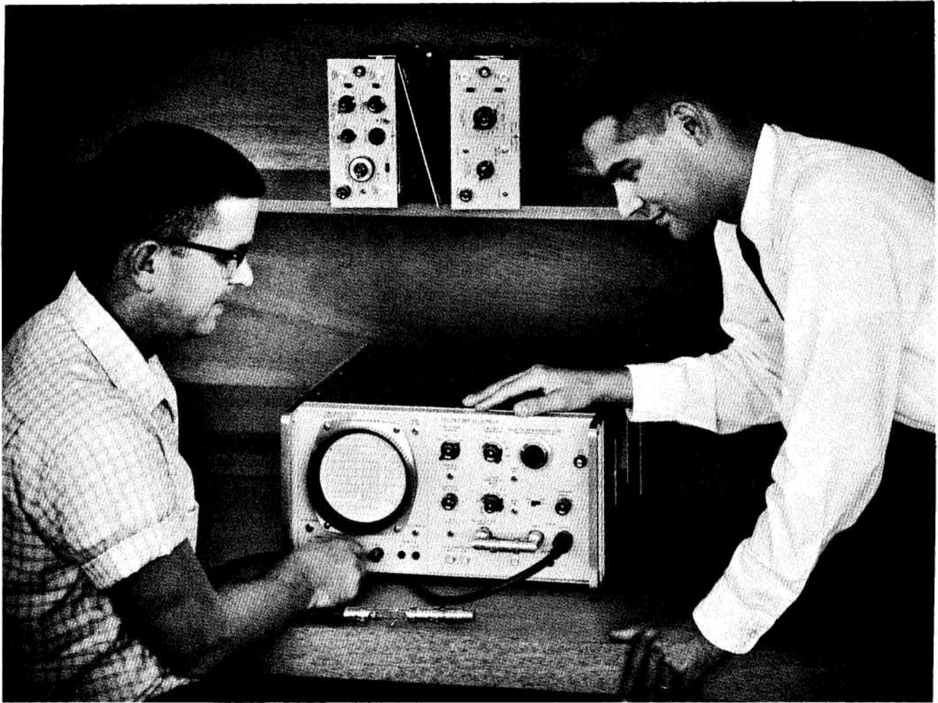
Time Domain Reflectometry, illustrated in the photo above, is an extremely powerful technique for analyzing transmission systems. The basic principles of this technique are described in this Application Note, along with some suggestions for accurate measurements.
